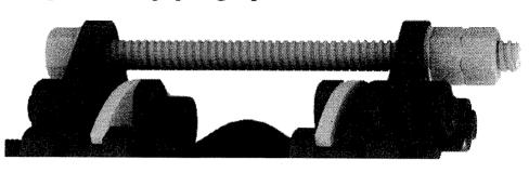
extend to a predetermined extension setting. Nuts shall be field-set to no more than the maximum allowable extension movement of a rubber expansion joint (unless used in an un-anchored system). Spherical washers can also be furnished (upon request) to combat any "nut-to-plate" binding during offset. **Consult the systems engineer** for proper nut settings prior to system operation.
