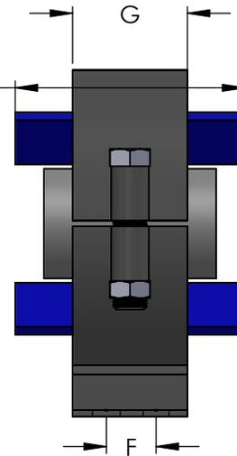
Spider Spacers Center Pipe In Housing And Are Sized To Allow Insulation To Be Packed Around Pipe
