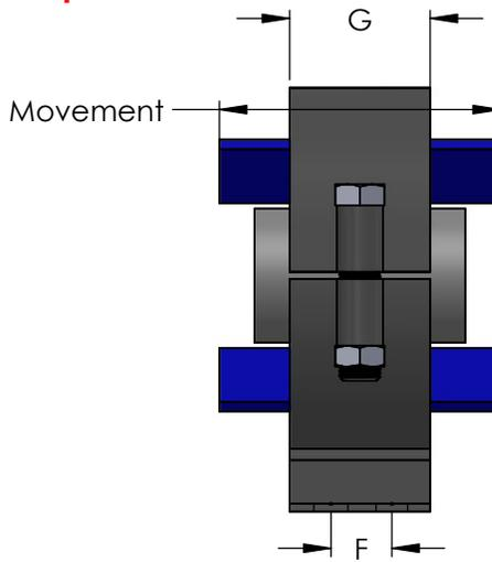
Spider Spacers Center Pipe In Housing And Are Sized To Allow Insulation To Be Packed Around Pipe
