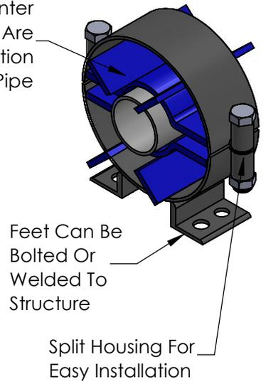
Provides Lateral Stability To The Pipe To Prevent "Bowling".
